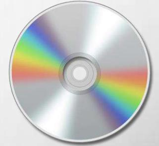
**3. Compact Disk – Read Only Memory** or CD-ROM is a read only or read-write disk. It can store large amount of data which can be distributed to large number of users. It is inexpensive and fast, but its access time is longer than that of magnetic disk.
